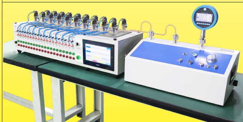
Verification of pressure switch calibration
